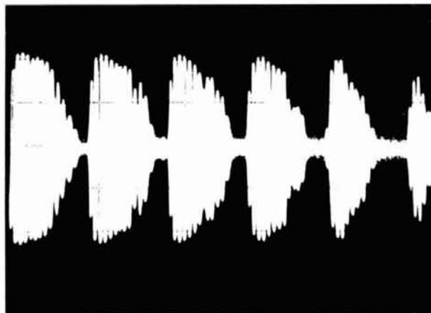
Transverter output on 80 meters showing ssb (upper) and CW (lower) modes as viewed on a Hewlett-Packard model 182 oscilloscope.
